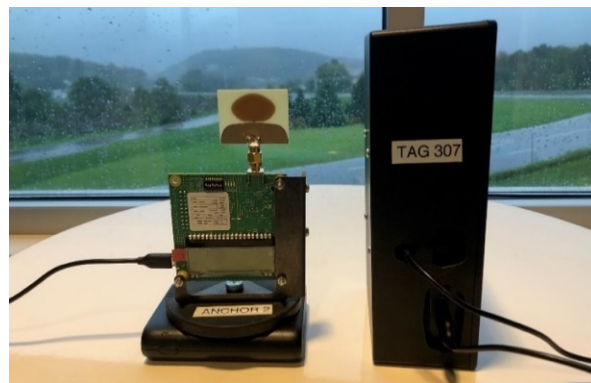
Figure 1. A picture of the DecaWave anchor tag setup (left) and mobile tag setup in the plastic enclosure (right).
