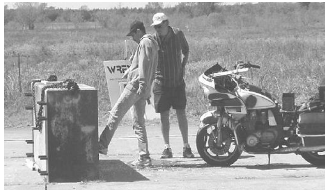
Figure 31. Concrete barrier and motorcycle type used in full-scale motorcycle crash testing (Adamson et al., 2002).
