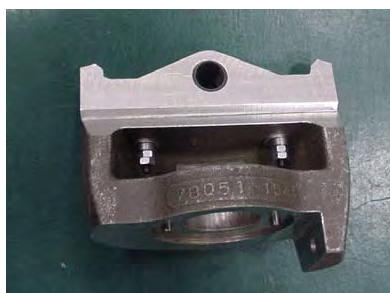
Figure 35. Frangible shoulder for Hybrid III dummy (Peldschus et al., 2007).
