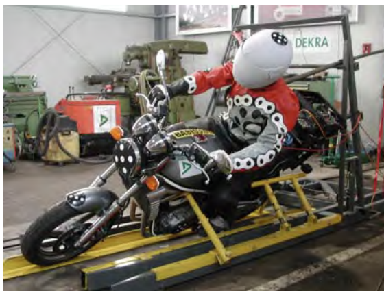
Figure 29. Test sled in inclined position with motorcycle and dummy (Peldschus et al., 2007).
