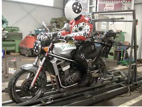
Figure 30. Test sled in upright position with motorcycle and dummy (Peldschus et al., 2007).
