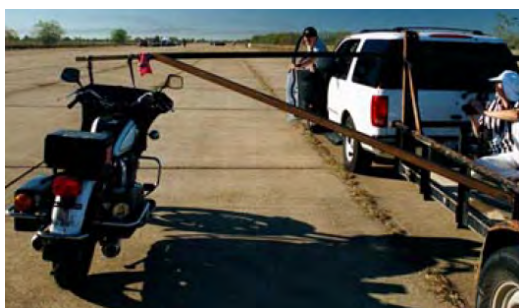
Figure 32. Motorcycle tow system (Adamson et al., 2002).
