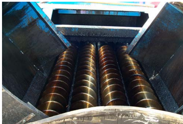
Photo 19. Auger system within the Novapaver.
