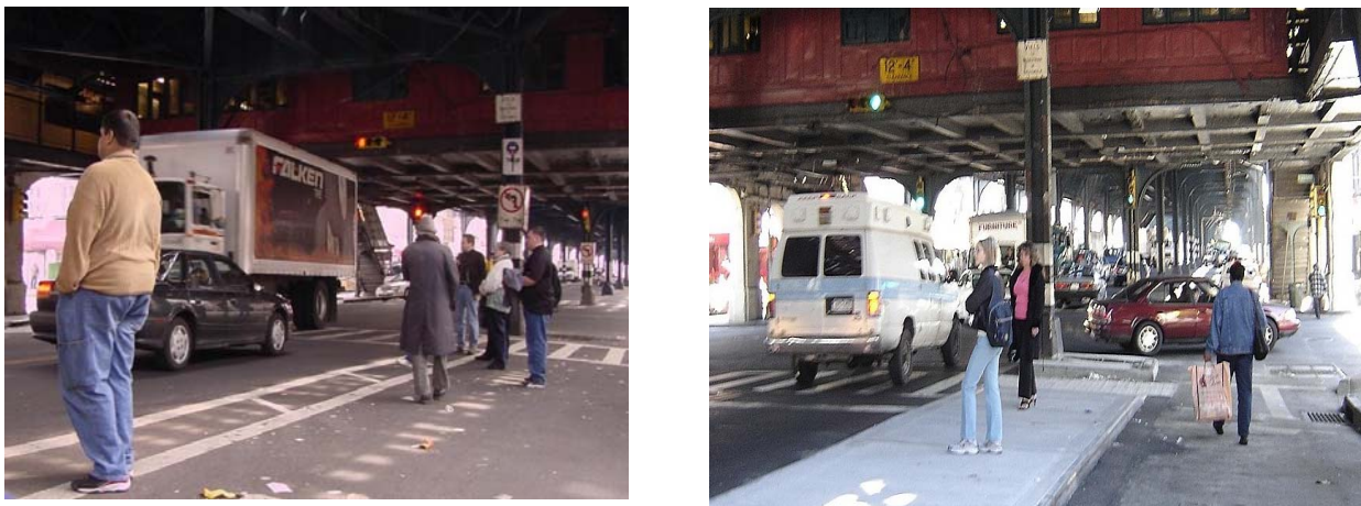
Figure 5.22 Bus Stops below Subway Tracks without and with Raised Median
