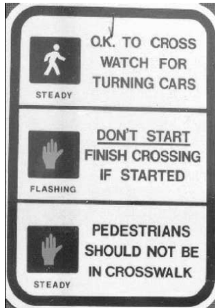
Figure 5.15 Sign to Explain Signal Designation
