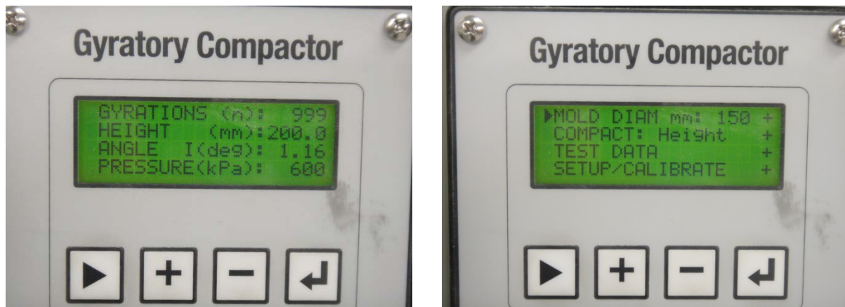
Figure 4. Compaction Parameters in Pine AFG2 Gyratory Compactor.
