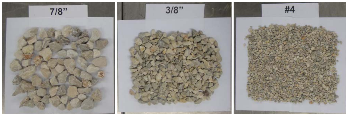
Figure 27. Aggregate Particles Used for AIMS Test.
