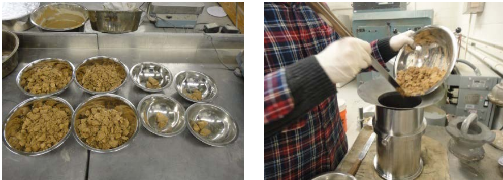
Figure 5. Sample Preparation of Base Material.
