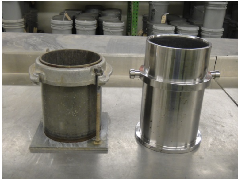
Figure 3. Molds for Impact Hammer and SGC Compactions.
