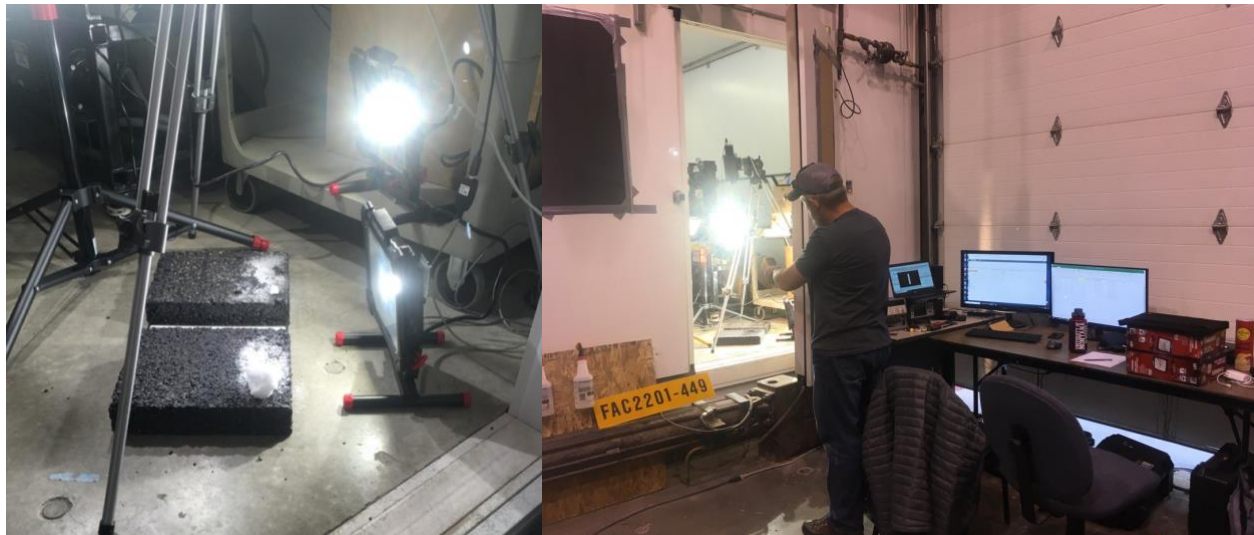
Figure 21: Experimental setup at MSU. The camera and asphalt samples were in the temperature-controlled room while data collection happened outside the room. Sample and room temperatures were recorded with each image.
