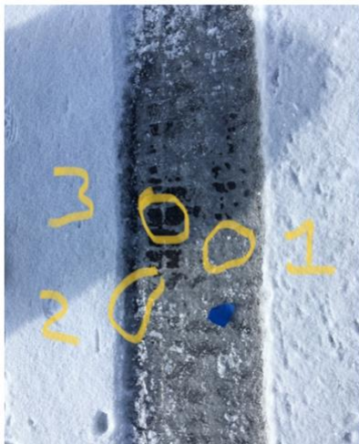
Figure 37: RGB photo of tread. Area 1 is ice, Area 2 has an area of black ice, and Area 3 is dry asphalt.
