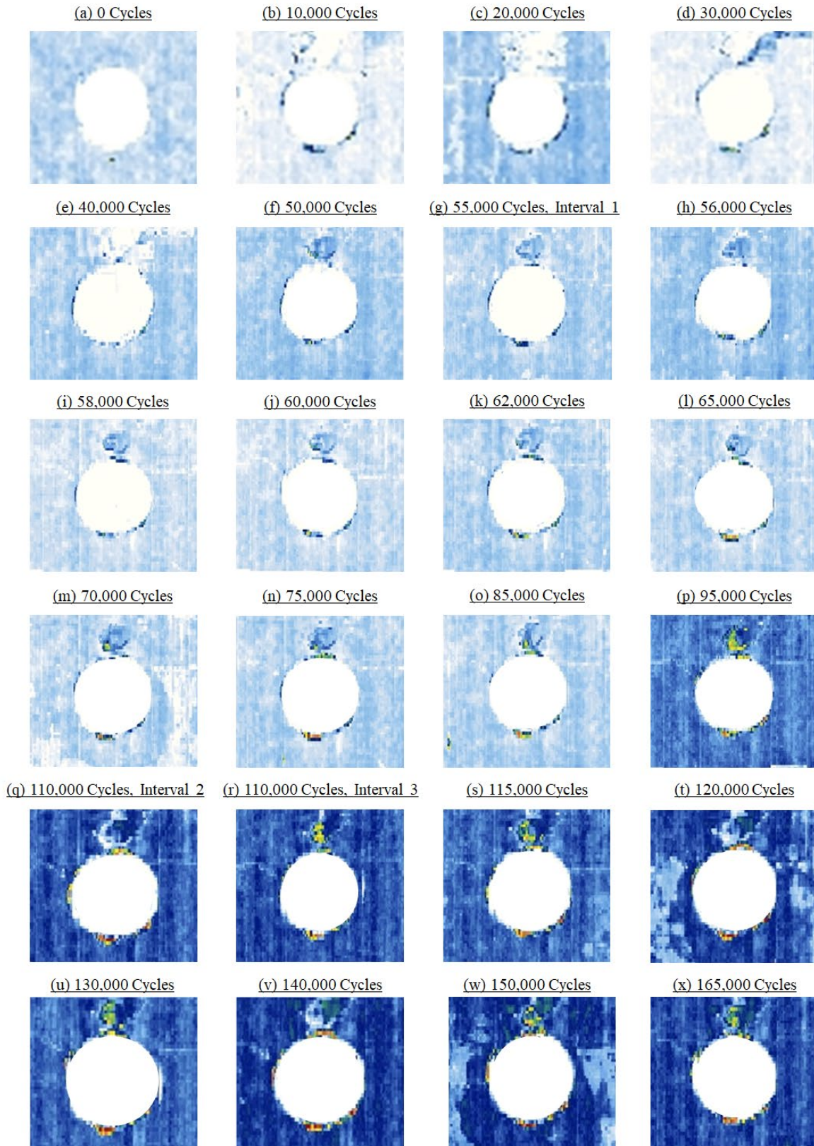
Figure 154. Phased array ultrasonic results (amplitude) for panel 2 throughout fatigue
