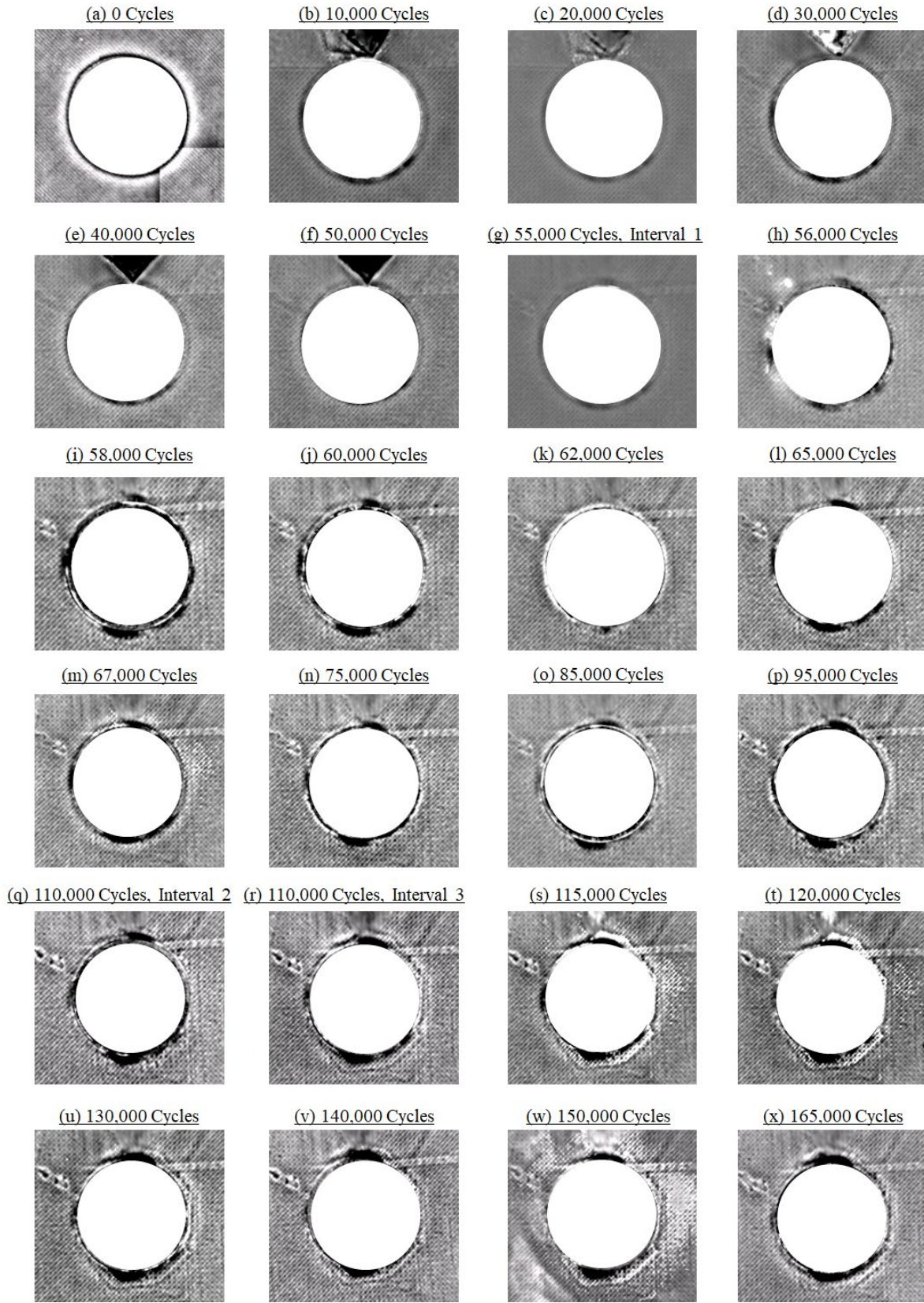
Figure 152. Flash thermography results captured for panel 2 throughout fatigue
