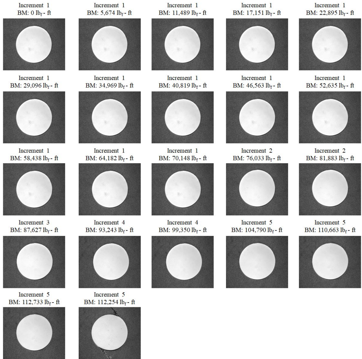
Figure 149. Panel 2 residual strength test, visual results by the left facing NFOV camera
