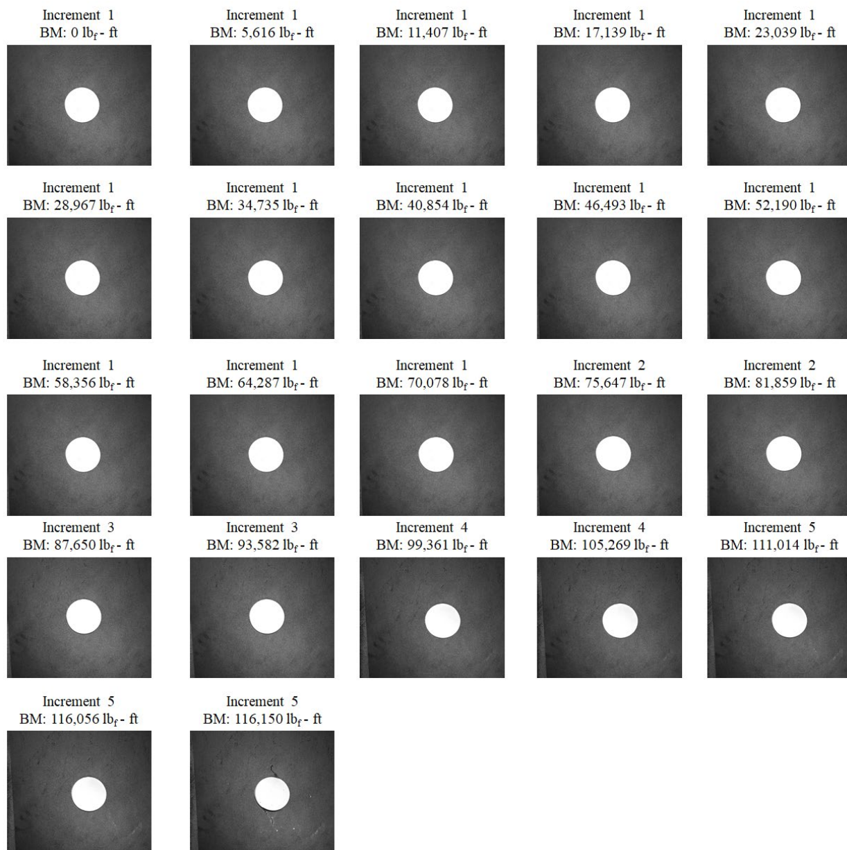
Figure 150. Panel 2 residual strength test, visual results by the left facing WFOV camera
