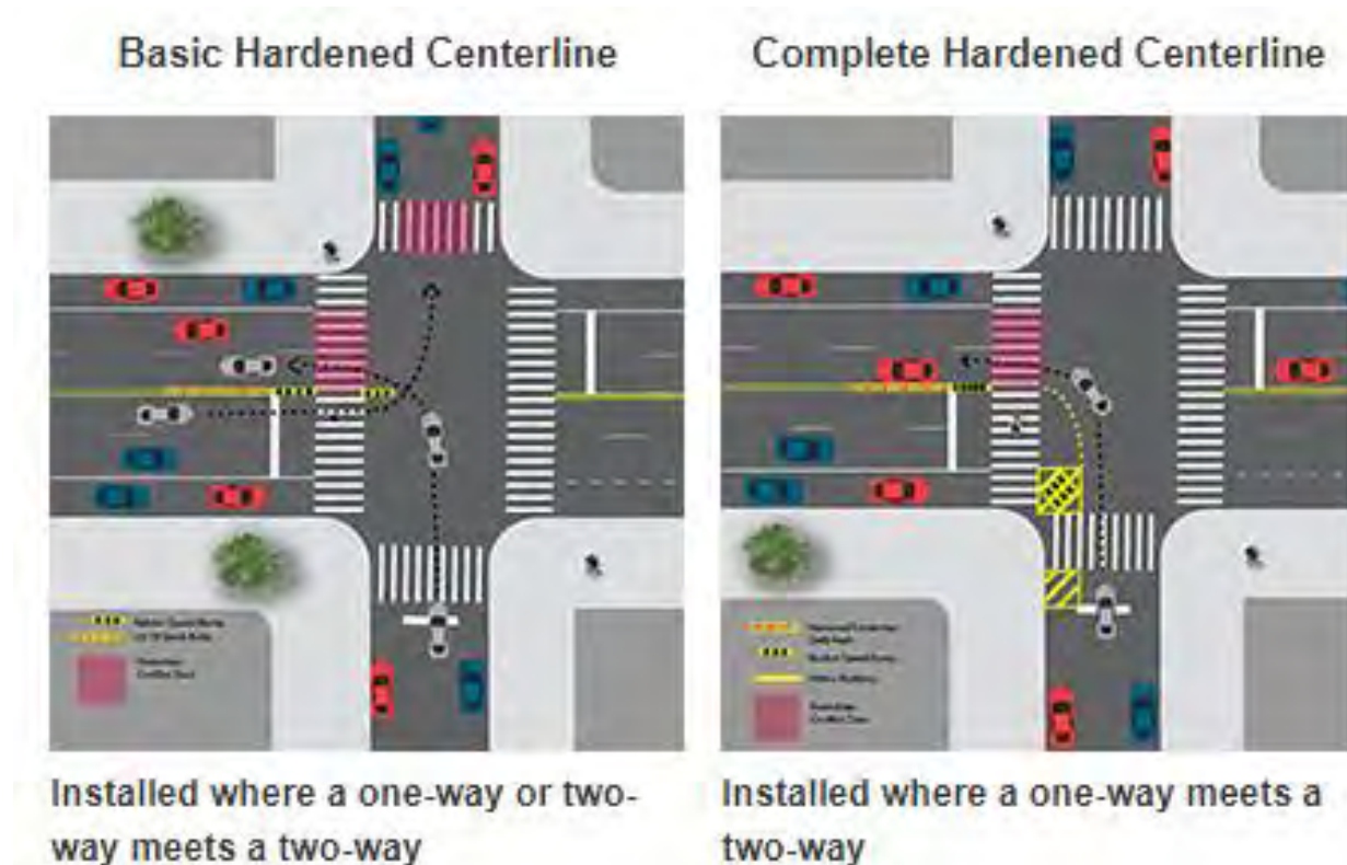
Figure 43. Drawing of Hardened Centerlines as Employed by New York City [A.113]
