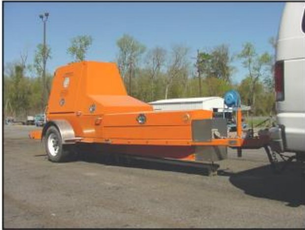
(a) Falling weight deflectometer (FWD)
