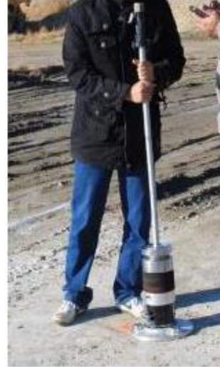
(b) Light falling weight deflectometer (LFWD), DYNATEST
