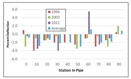
Figure 1: 24 Inch Pipe, East End, Station 361+25
