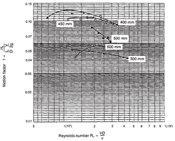
Figure 9.14 Diagram of Darcy-Weisbach friction factor vs. Reynolds number for diameter of pipes as indicated.
