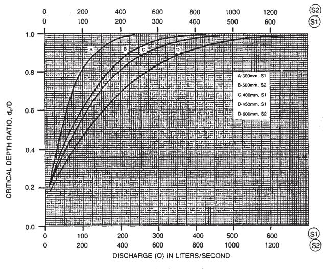
Figure 9.15 Critical depth of flow in Big 'O' heavy duty pipes.
