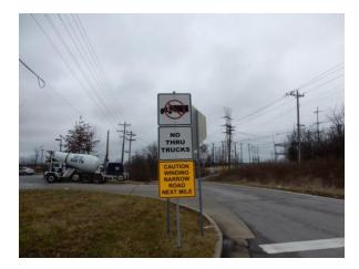
• **KY 1198 in Bath County:** A version of a truck prohibition sign was installed to limit commercial truck traffic on a road where the geometrics were inappropriate for large trucks.
