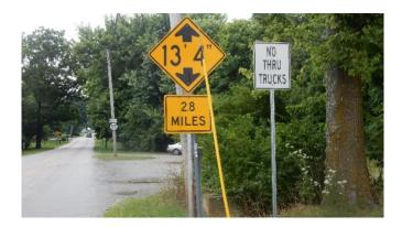
• The following images are examples of truck prohibition signs used (primarily by counties and cities) on roads where truck drivers were led by GPS units onto inappropriate routes. Inspections have found a range of signs used, with many signs being either non-standard or installed improperly.
