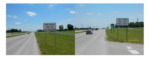
• **KY 57 in Bourbon County:** Truck drivers had been provided incorrect information for the proper route to make a delivery. This resulted in large trucks traveling on a route with a height limitation and drivers being forced to turn around in a parking lot, resulting in damage to the property. Warning and regulatory signs were installed to stop the drivers before they reached the low overpass. However, drivers continued to have problems due to the routing directions.
