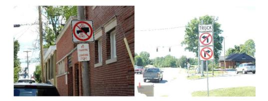
• A warning sign was installed to advise truck drivers of a change in the road configuration and specifically told drivers to reprogram their GPS units.
