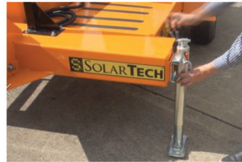
(b) Jacks being deployed to stabilize the base of the mast
