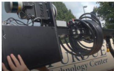
(c) TScan head unit being mounted to the mast
