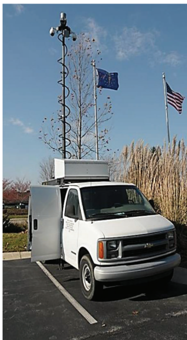
Figure 3.1 Mobile traffic laboratory with TScan hardware.
