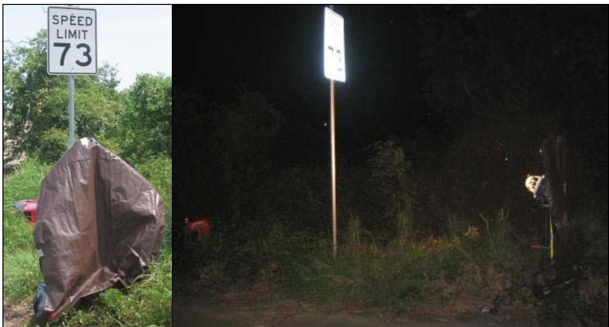
Figure 9. Floodlight on Sign 11 at Day and Night.
