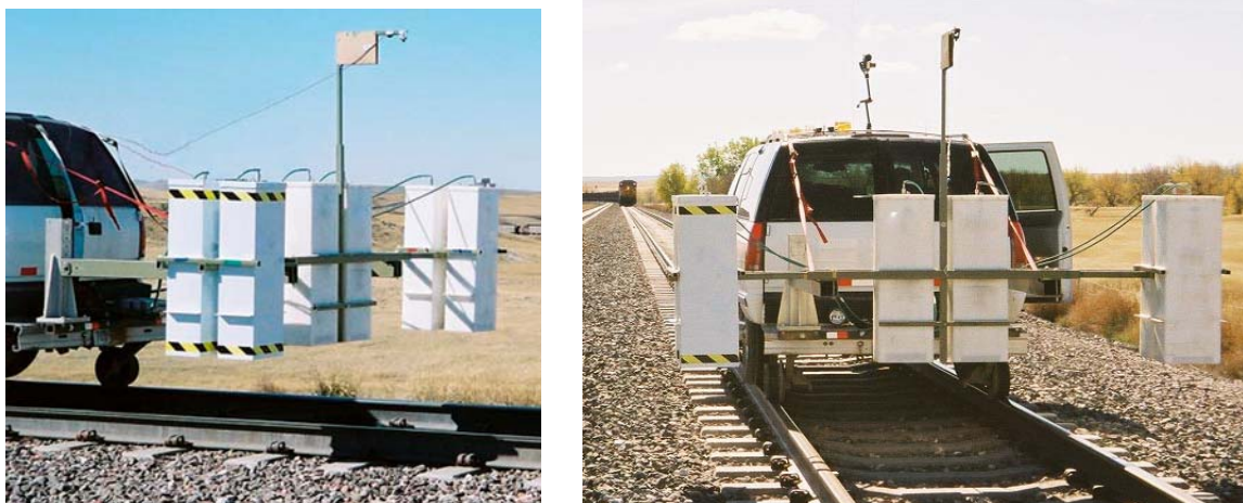
Figure 1. GPR Test Equipment Deployed for Track Inspection
