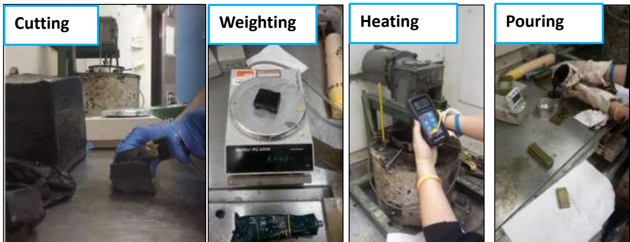
Figure 18 Main steps followed in crack sealant sample preparation
