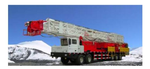
Figure 42 XJ 550 truck mounted workover rig
