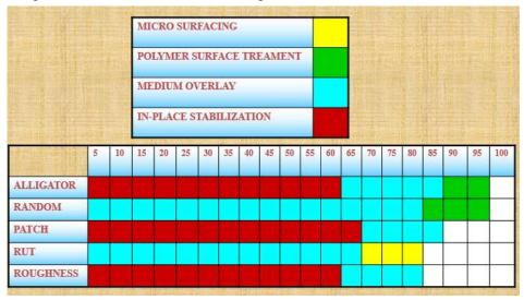
Figure 32 Pavement maintenance triggers and distress index
