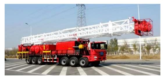
Figure 40 ZJ 10/900CZ truck mounted drilling rig
