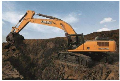
Figure 51 Case CX470B excavator
