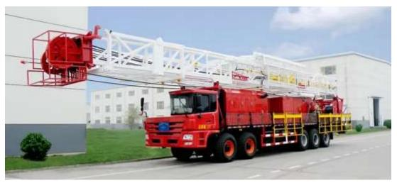
Figure 41 XJ 350 truck mounted workover rig
