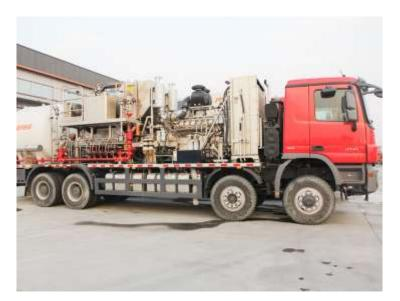
Figure 49 Weber trailer mounted 180K N2 pumper
