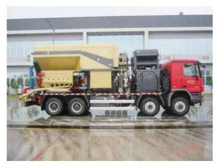
Figure 44 YLC140-5600 truck mounted fracturing unit
