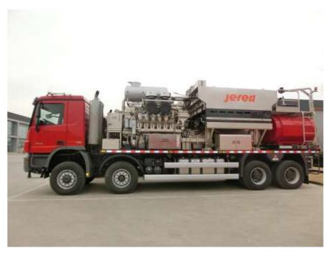
Figure 46 YLC105-2250 truck mounted fracturing unit
