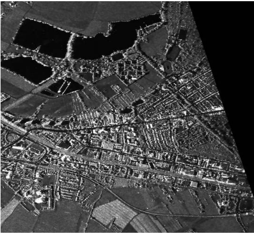
Figure 14: This is a very high resolution SAR image, of the same area in Figure-11, acquired with airborne ESAR that has the same (1-5 meter) resolution as the TerraSAR-X satellite.
