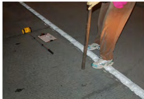
Sounding of delaminated area with no superficial distresses
