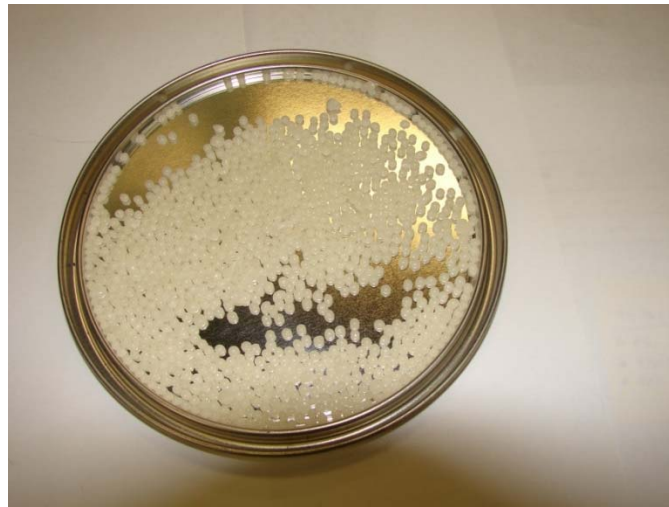
Figure 6 Pellets of the chemical additive Sasobit
