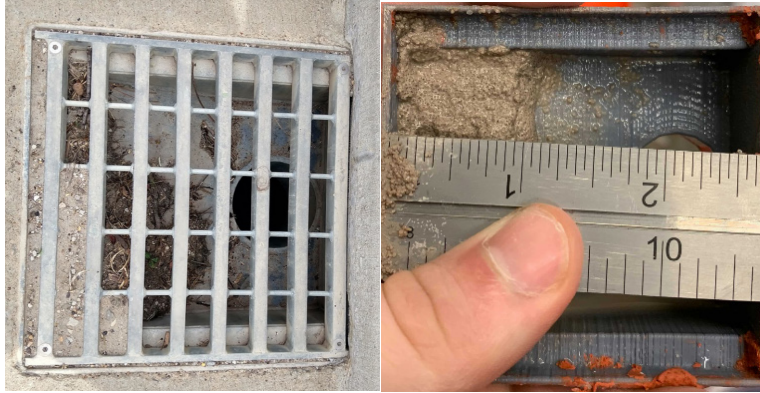
Figure 4.7: Clogged Inlet (Left); Simulated Experimental Mix (Right)
