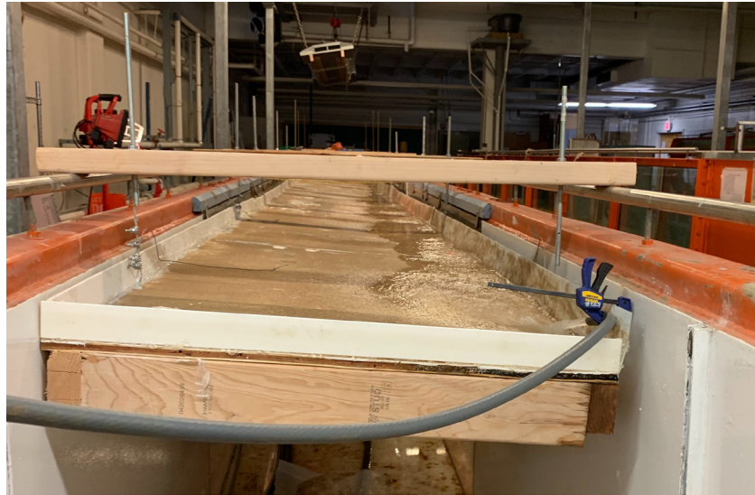
Figure 4.3: Single Inflow from High Side of Scale Bridge Deck Model
