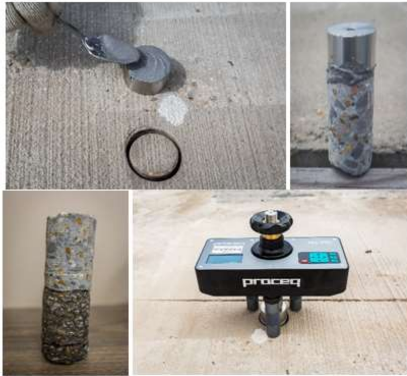
Figure 36 Tensile bond strength test on BCOA sections
