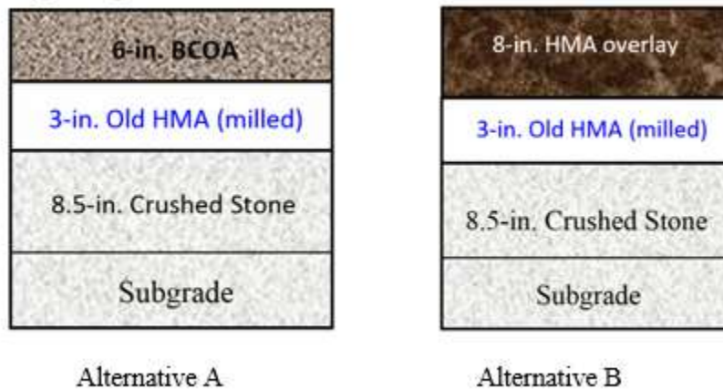
Figure 30 Pavement alternatives used in cost-benefit analysis
