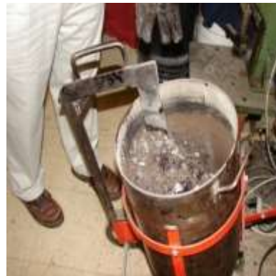
Asphalt binder and aggregate mixed together
