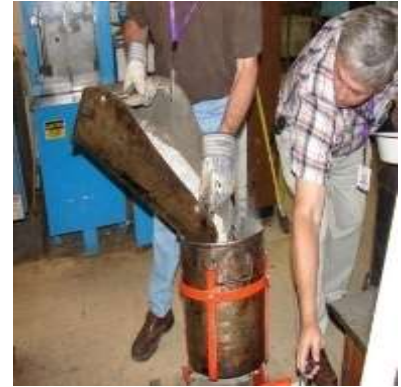
Superheated aggregate placed on top of RAS and/or RAP
