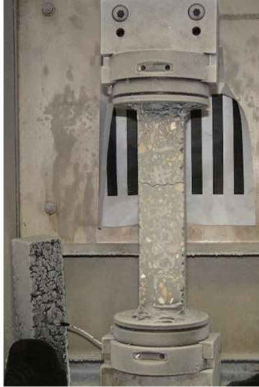
Figure 18 TSRST test setup and thermally fractured specimen
