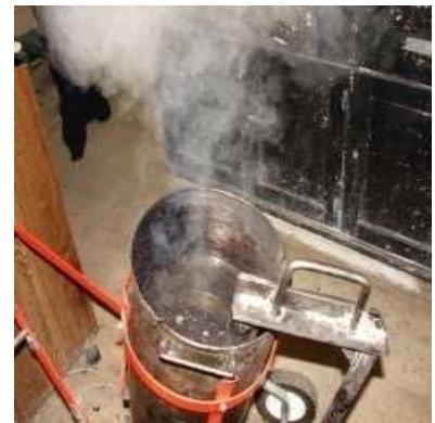
Steaming occurs during initial mixing. After mixing, back in oven till aggregate blend achieves mixing temperature
