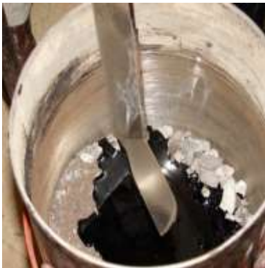
Asphalt binder added to prepared aggregate blend
