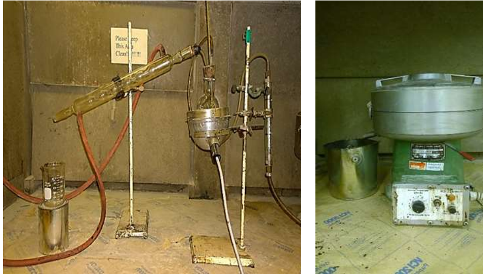
Figure 2 Centrifuge and Abson test setup
