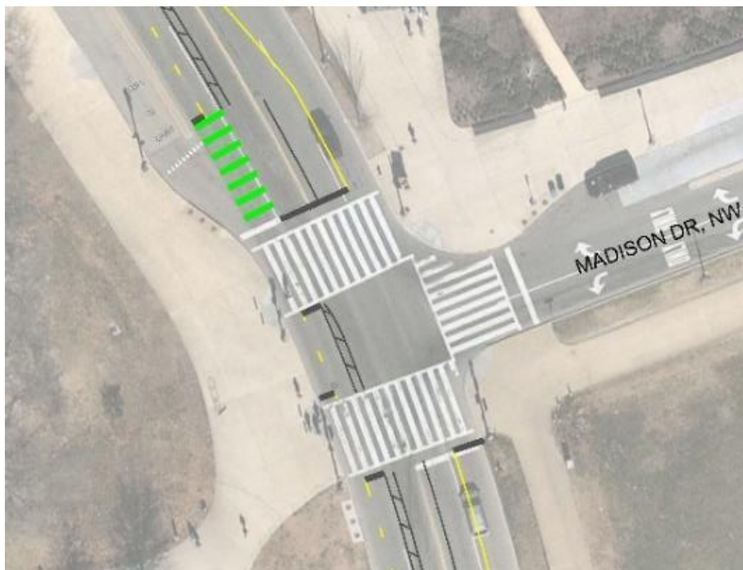
FIGURE 2: CONCEPTUAL DESIGN FOR CYCLETRACK AT INTERSECTION OF 15 TH STREET AND MADISON DRIVE (NELSON\NYGAARD, 2020).
