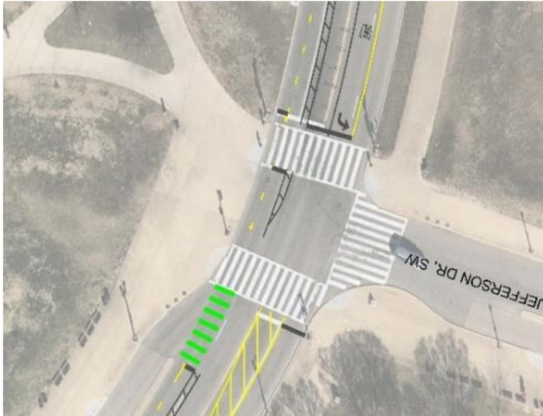
FIGURE 3: CONCEPTUAL DESIGN FOR CYCLETRACK AT 15 TH STREET AND JEFFERSON DRIVE (NELSON\NYGAARD, 2020).
