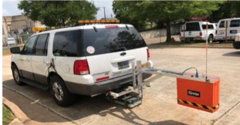
Figure 42. Description of the GPR testing setup
