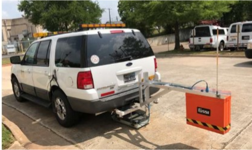
Figure 16. Layout of a GPR system
