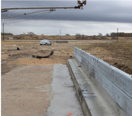
(a) Bridge rail/test vehicle after test
