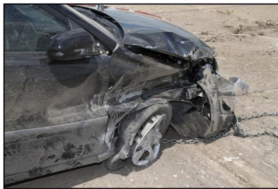
(b) Damage to right front tire
