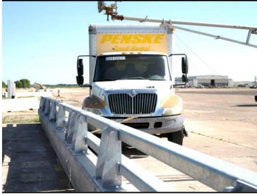
(a) 10000S test vehicle at impact point
