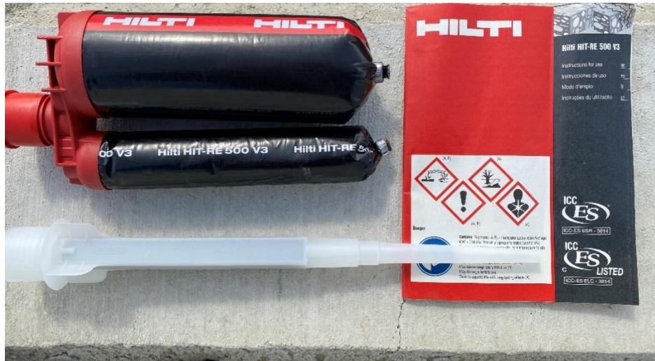
Figure 93. Hilti HIT-RE500-V3 Adhesive Anchoing System used (anchor bolts installed as per manufacturer's specifications)
