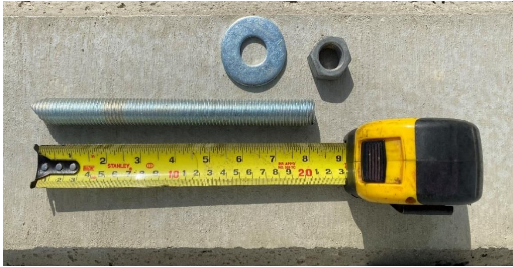
Figure 92. Hot dipped A193 B7 ¾-in. diameter Hilti threaded rod
