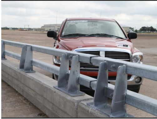
(a) 2270P test vehicle and bridge rail
