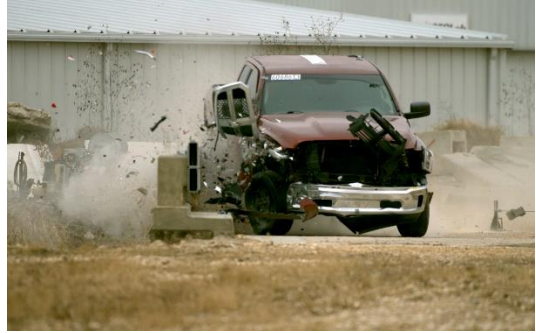
Figure 130. Sequential photographs for Test No. 606861-3 (frontal view).
