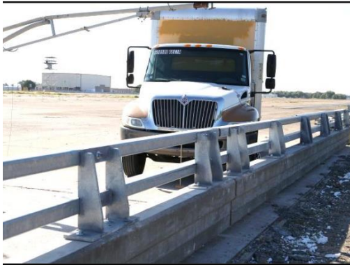
(a) 10000S test vehicle and bridge rail
