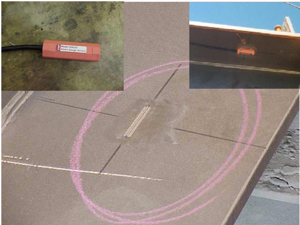
Figure 2-33: Steel strain gage and reader. Clockwise from upper left: reader, gage and reader in place, gage after being placed on reader.
