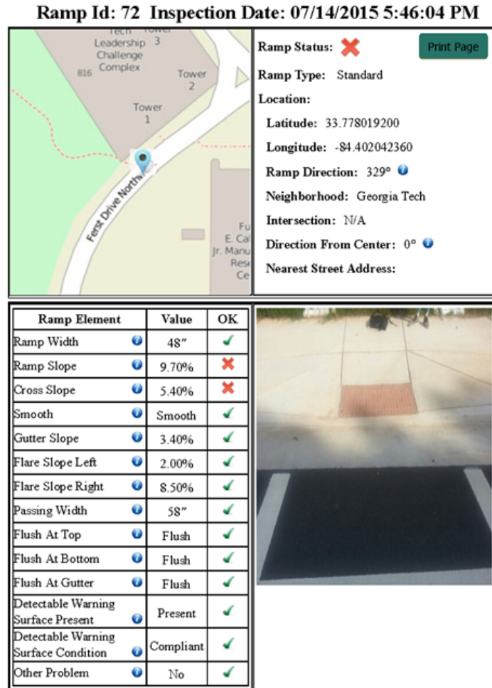
Figure 9. Example of a Semi-Static Dashboard for Individual Ramp Field Inspection Results
