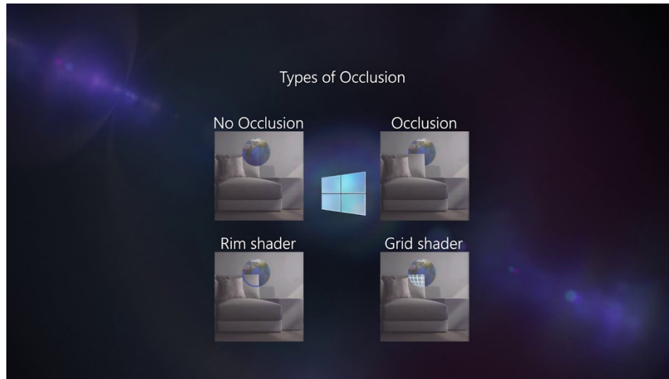
Figure 33: Types of Occlusion available in Unity3D + HoloLens setup
