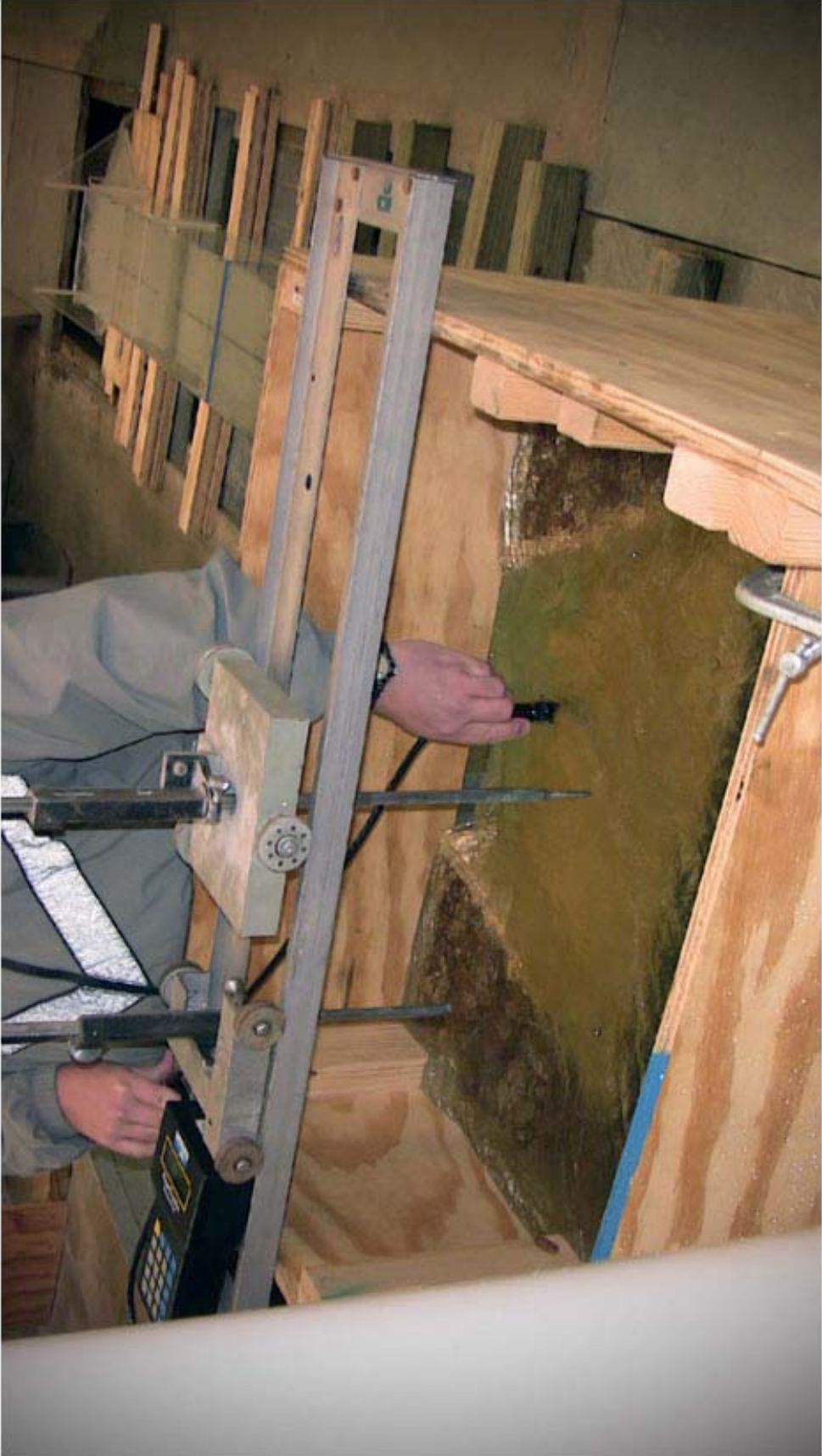
Figure 13. Reservoir with point gage to measure water level.
