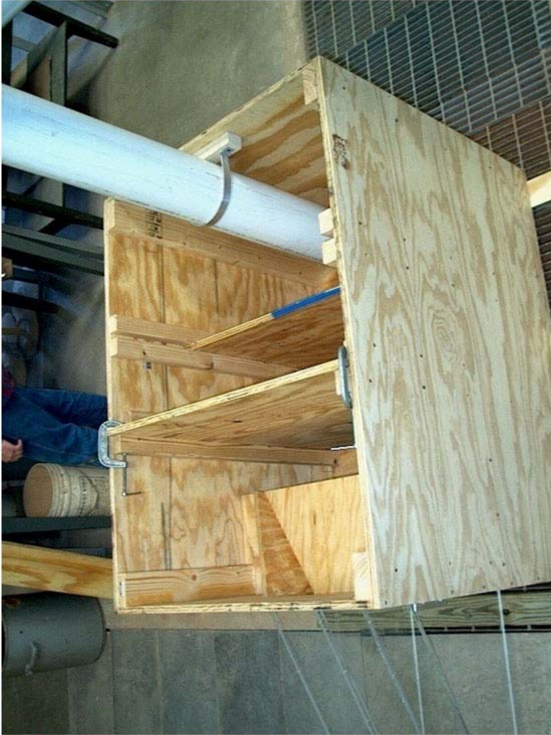
Figure 12. Reservoir and channel inlet for culvert model.
