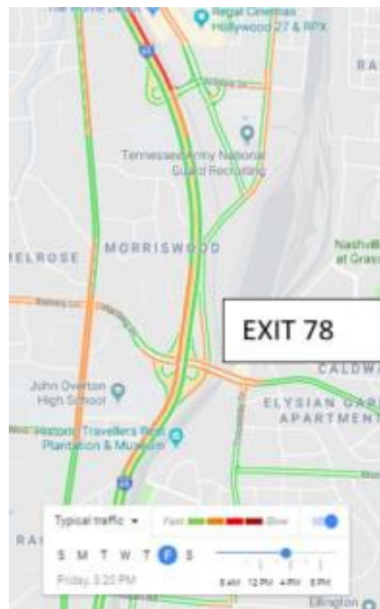
Figure 9-11 Google Traffic data showing queue spillback from Exit 78
