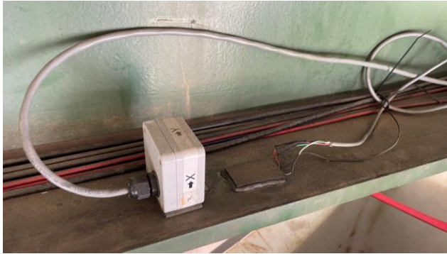
A. Integrated accelerometer and covered strain gage.
