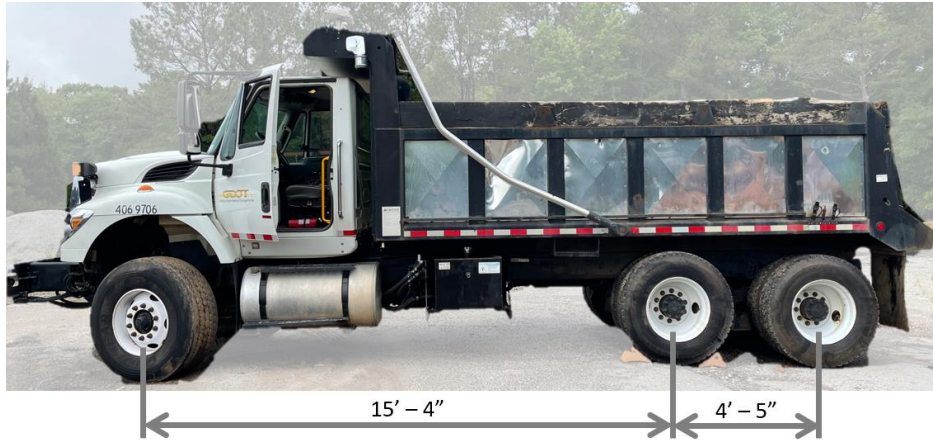
Figure 11. Photo. GDOT dump truck with axle spacings dimensioned.
