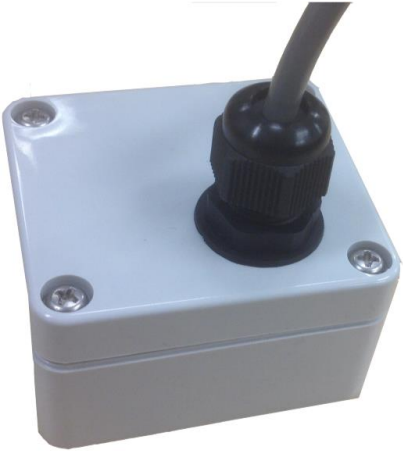
B. Weatherproof case enclosing the accelerometer board.
