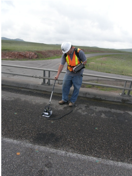
Figure 2 - Ingegneria Dei Sistemi (IDS) Aladdin acquisition system with a full-polar 2000 MHz antenna and Panasonic Toughbook CF-19.
