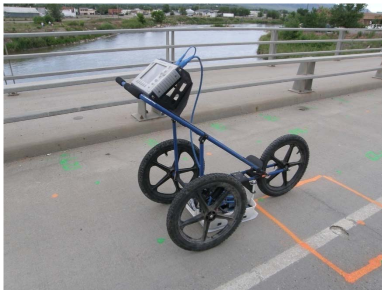
Figure 10: Typical GPR ground-coupled cart.
