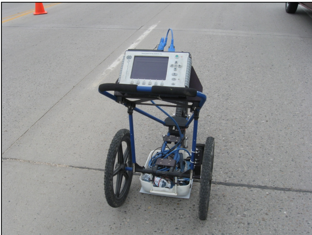
Figure 2 - SIR-3000 GPR system with a 1500MHz ground coupled antenna mounted on a cart.
