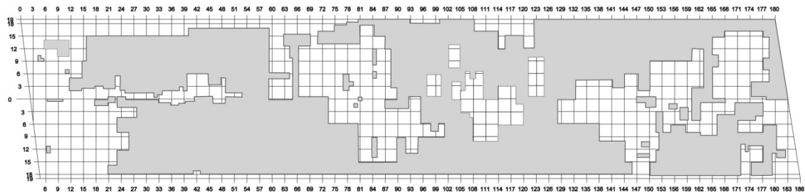
Figure A.24: Chain drag results outlining areas of delaminations
