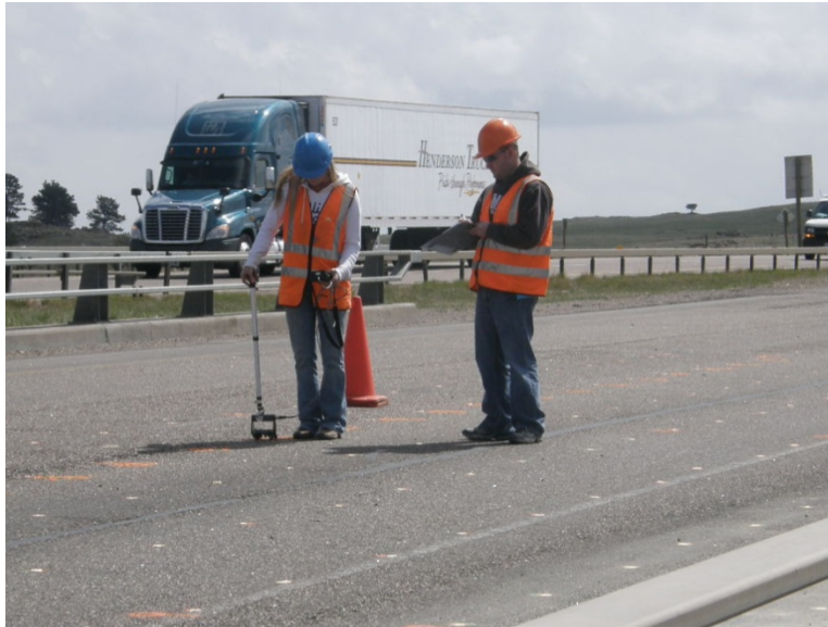
Figure 18: University of Wyoming researchers performing impact echo test.
