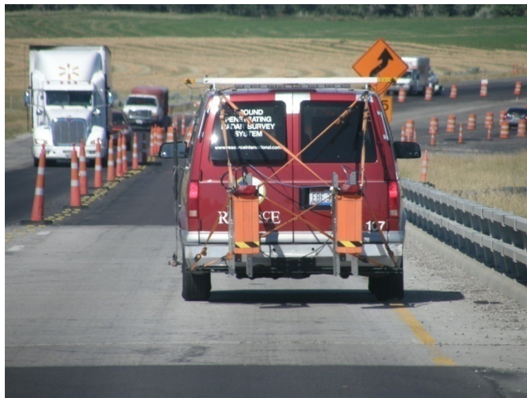
Figure 29: Rii's van-mounted system scanning the bridge.
