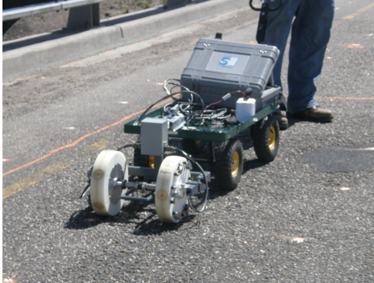
Figure 5: Olson Engineering's Impact Echo Bridge Scanner.
