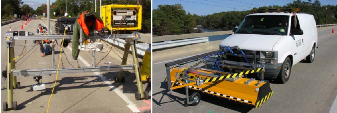
Figure 9: PERES II system and vehicle mounted systems (Huston et al. 2007b).
