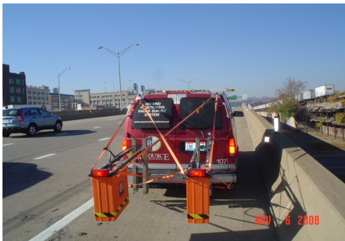
Photograph 2. GPR vehicle used during data collection
