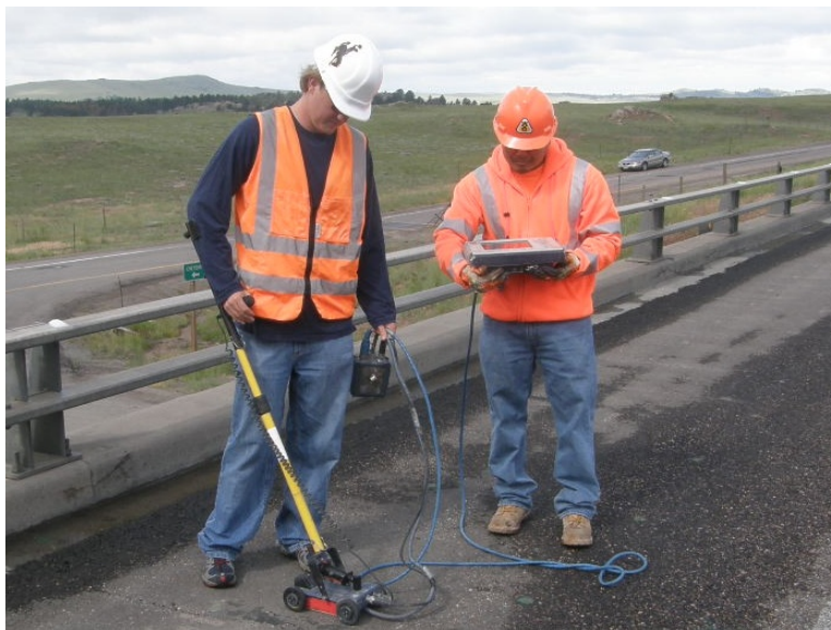
Figure 23: Ground-couple GPR system without cart.
