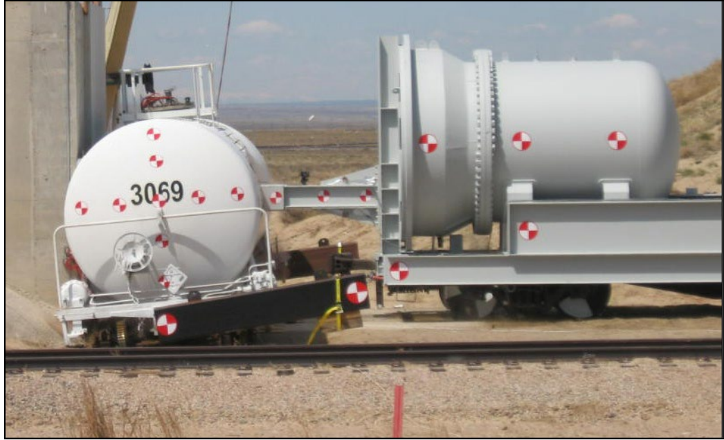
Figure 17. Test 1 – Shell Side Impact Behavior in Test 1 for Tank Car 3069
