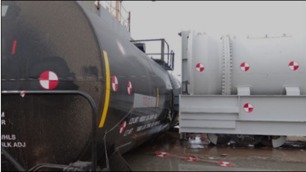
Figure 39. Test 4 – Post-test Puncture Response of the Tank Car
