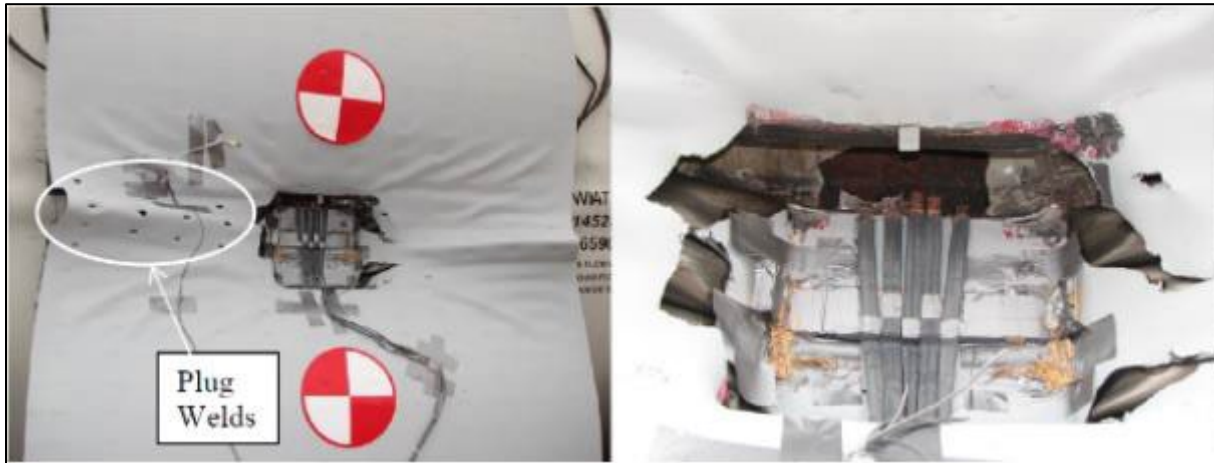
Figure 33. Test 3 – Damage to Protective Panel
