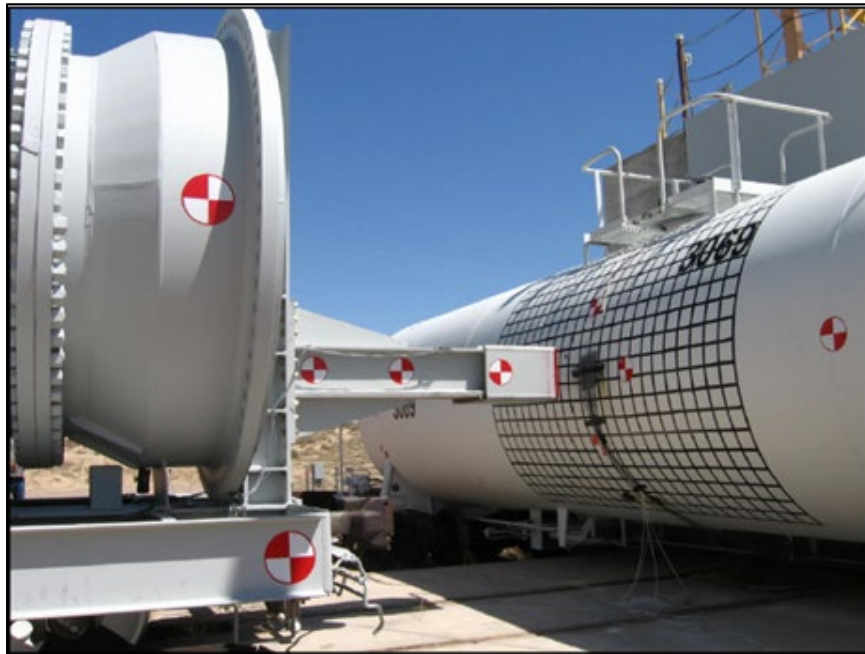
Figure 16. Test 1 – Test Setup Showing Tank Car
