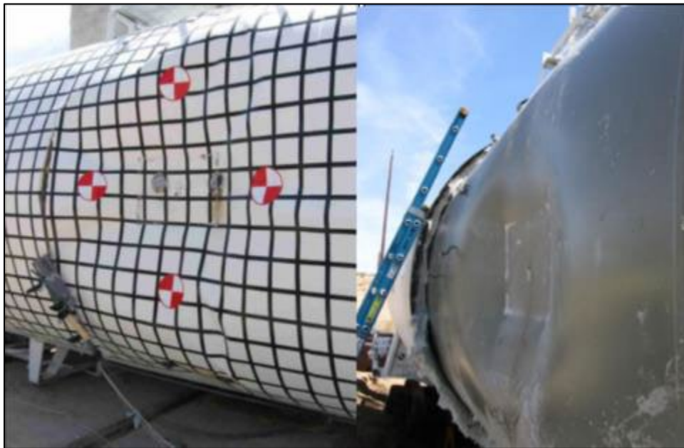
Figure 18. Test 1 – Post-Test Dents in the Jacket and Shell of Tank Car 3069
