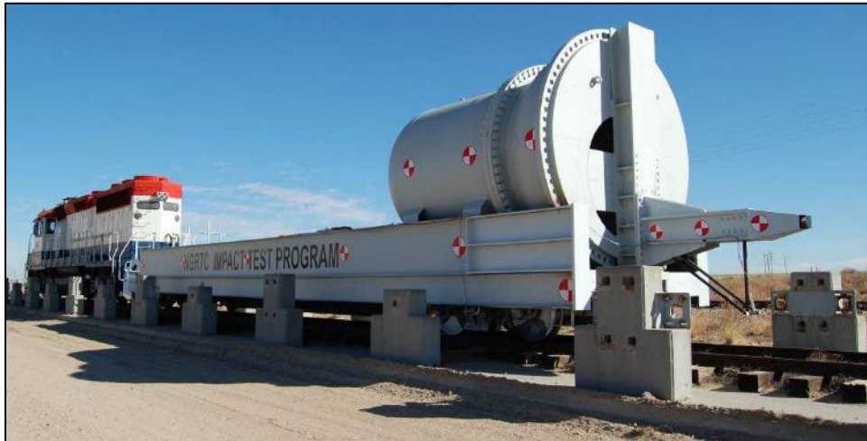
Figure 26. Test 2 – Modified Impactor Car and Impactor Head Used in Test 2
