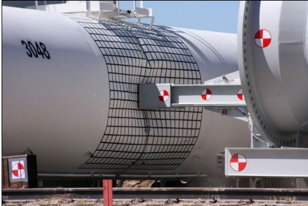
Figure 9. Test 0 – Impact Response (Near maximum impactor displacement)
