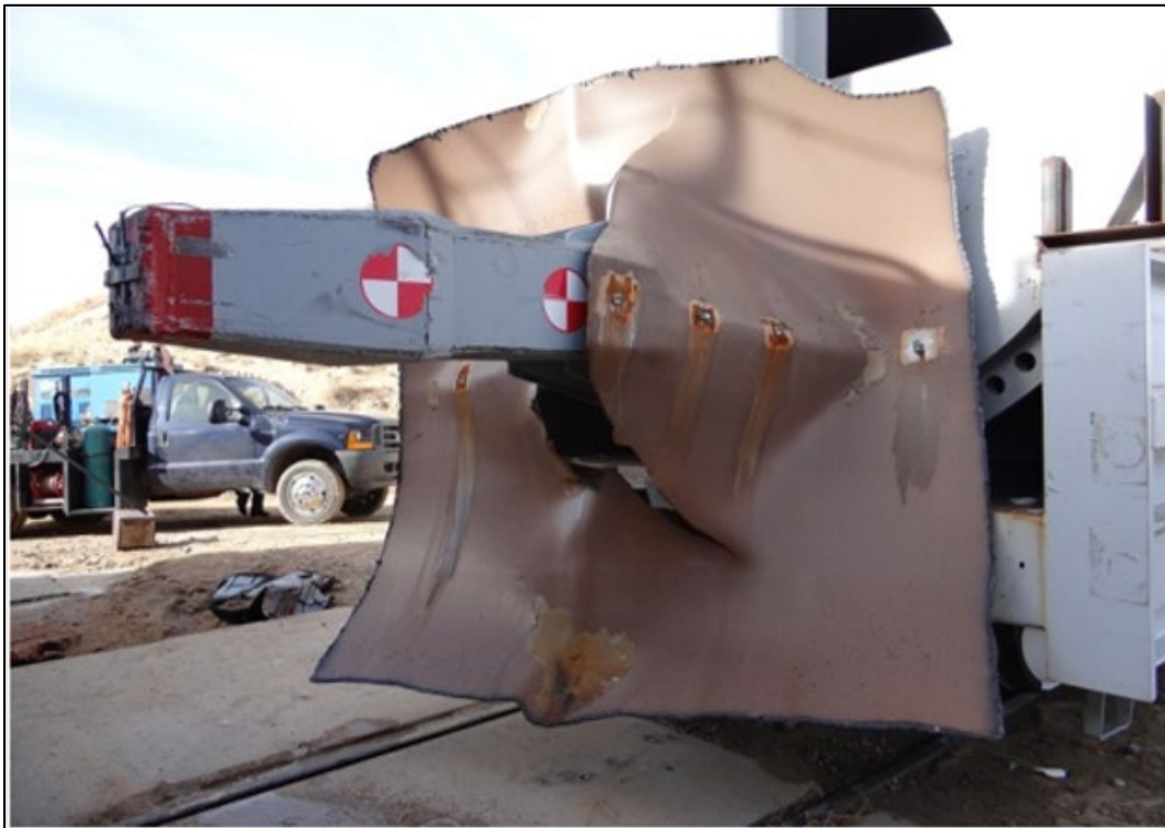
Figure 40. Test 4 – Post-test Puncture Damage of the Tank Car
