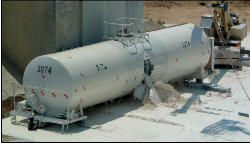
Figure 27. Test 2 – Puncture Response Observed in the Full-Scale Impact Test 2
