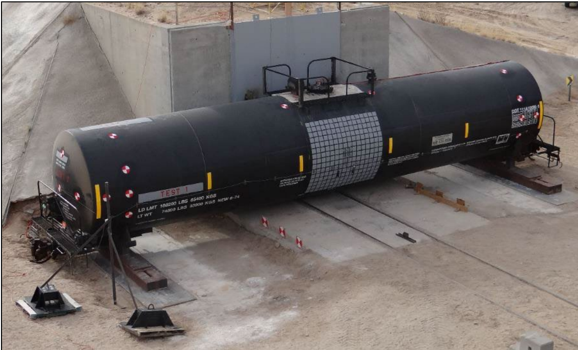
Figure 36. Test 4 – Target Tank Car Mounted on Support Skids
