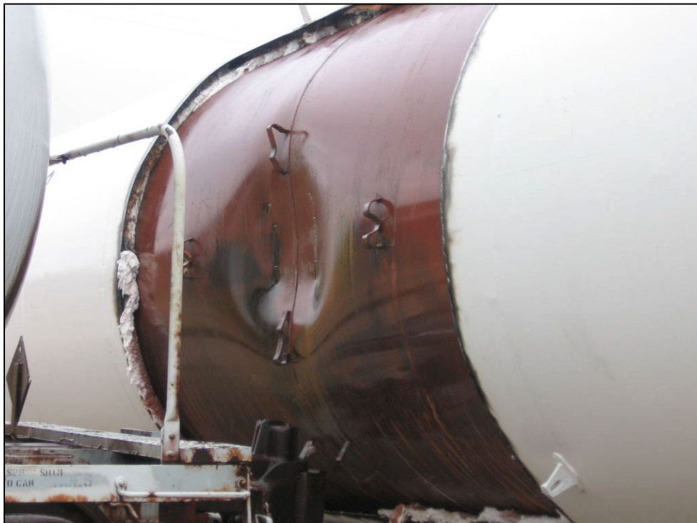
Figure 10. Test 0 – Impact Damage to the Inner Tank Shell
