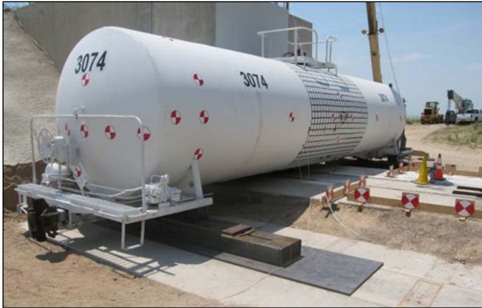
Figure 25. Test 2 – Tank Car 3074 Mounted on Support Skids
