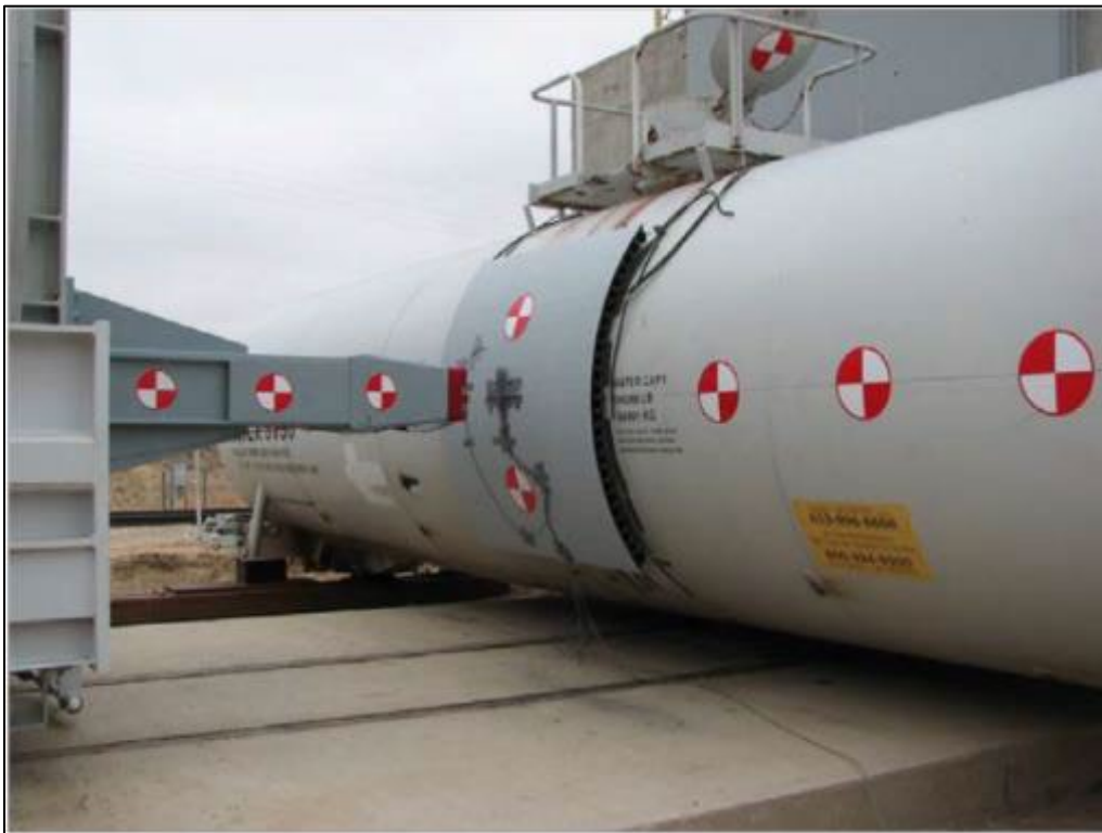
Figure 32. Test 3 – Test Setup Showing Tank Car and Impactor
