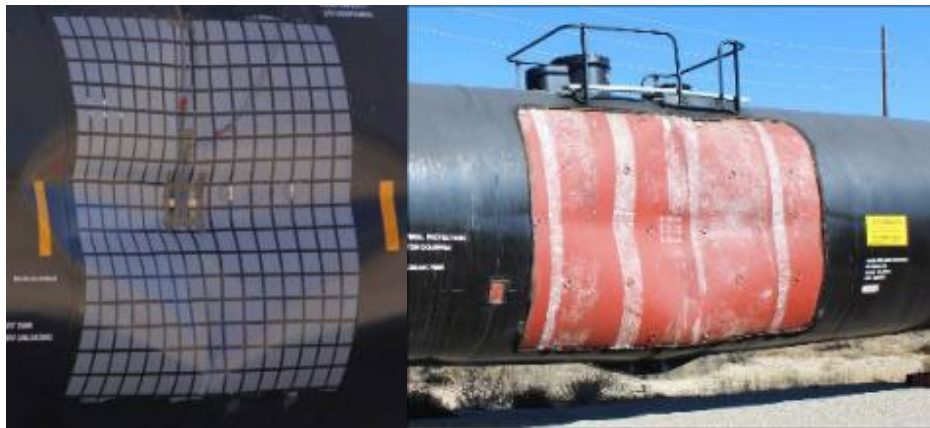
Figure 59. Test 7 – Post-test Images of (left) the Tank Car with Jacket and (right) Tank Inner Shell
