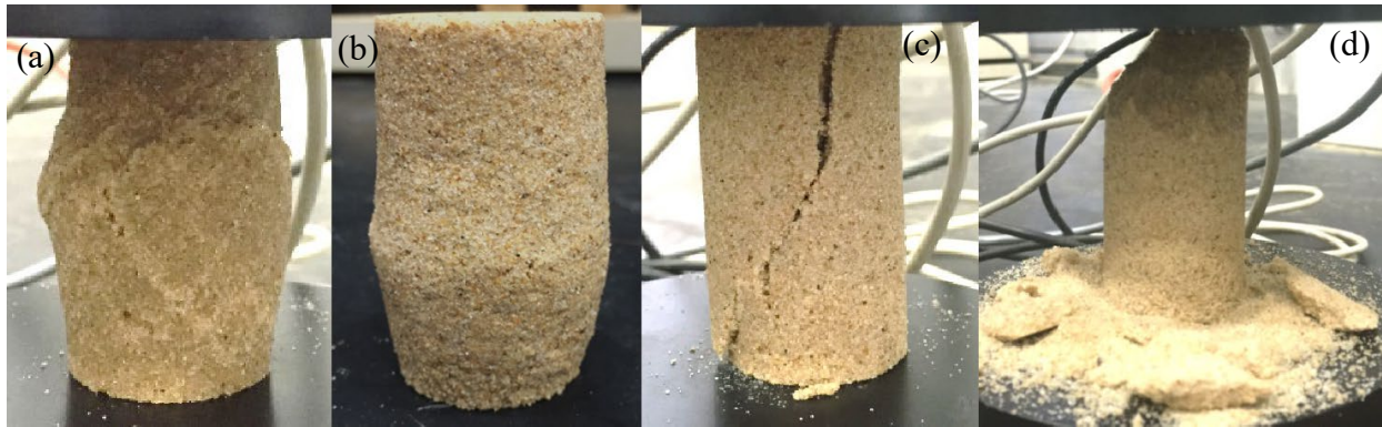
Fig. 9 The failure mode of hydrogel-impregnated sand under (a) wet condition; (b) air-dry condition; (c) 50°C oven-dried condition; (d) 100°C oven-dried condition.
