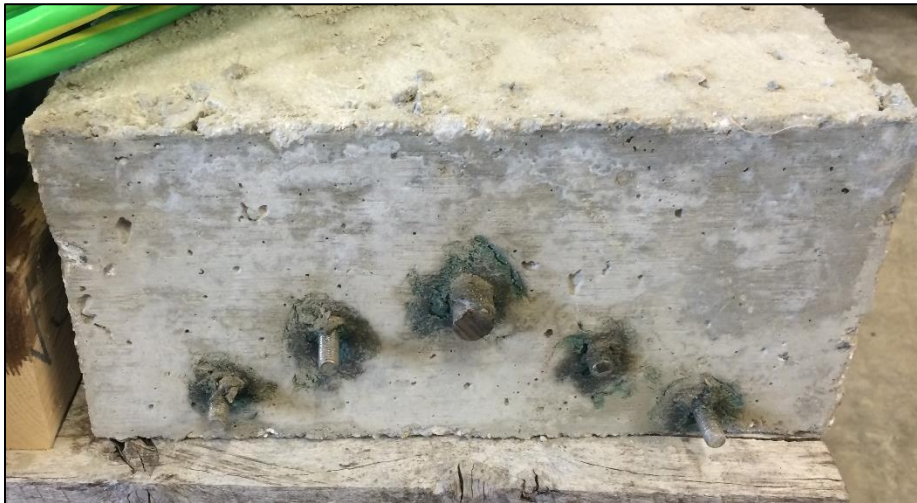
Figure 3.8: Photo of marine exposure block showing locations of reinforcing steel
