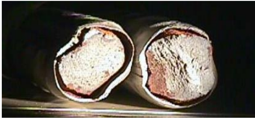
Figure 4.1: Stainless steel-clad bar failure following tensile test (Cross, et al. 2001)
