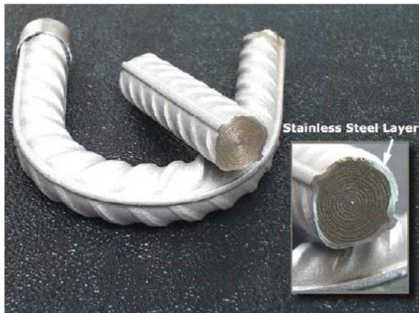
Figure 2.1: Stainless steel-clad reinforcement (Clemena, Kukreja and Napier 2003)
