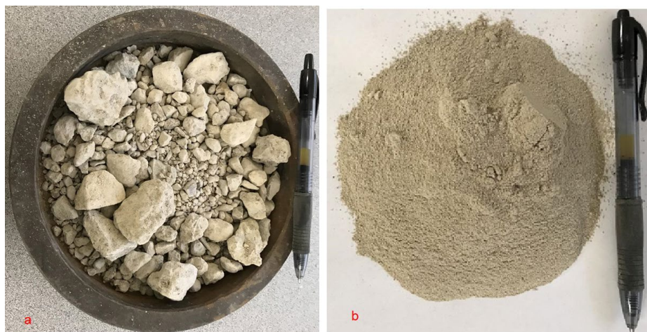
Figure 3.1.2 Sample Preparation for RCA pH and Chloride Analysis
