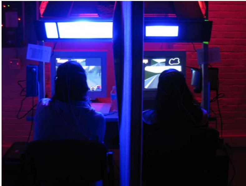
Figure 4: Driving simulator with subjects separated by a divider in the centre. The Left side subject is exposed to B2 while the right side subject is exposed to B1 light condition.
