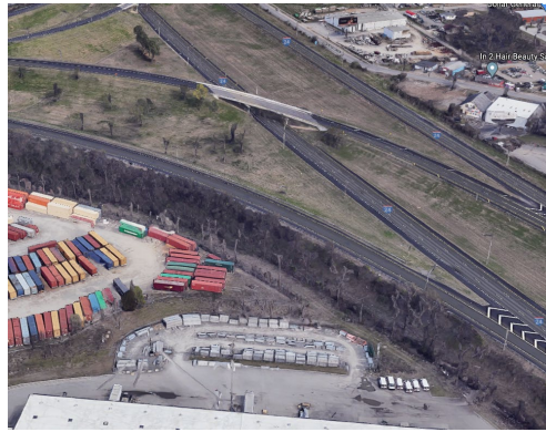
Figure A.4 Caveat of using Google Maps Elevation API for extracting the elevation a) 3D perspective of an unlevelled intersection b) 3D overview of the same intersection using the elevation extracted from Google Maps Elevation API
