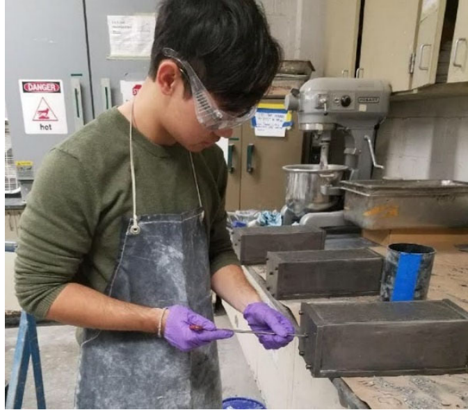
Figure 8-5: Prism demolding after initial curing
