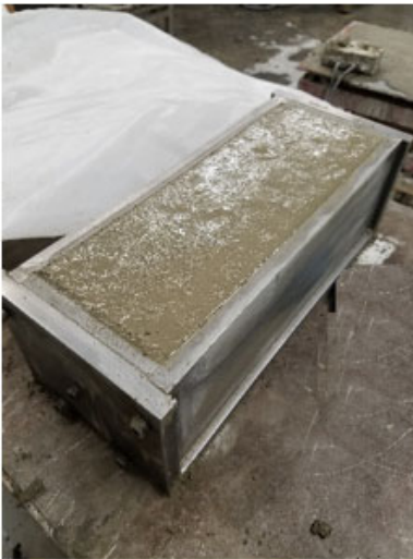
Figure 8-4: Sample after finishing
