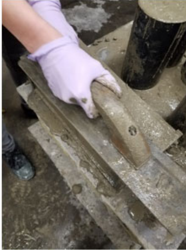
Figure 8-3: Prism being finished
