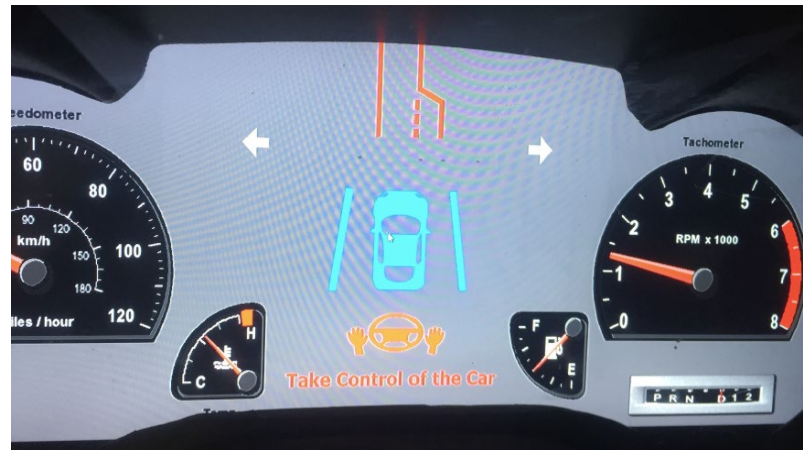
Figure 10. Advanced Dashboard for road geometry (Second iteration)
