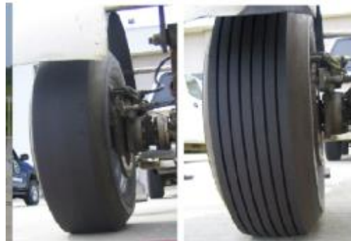
Figure A.23. Smooth vs ribbed tire (30).
