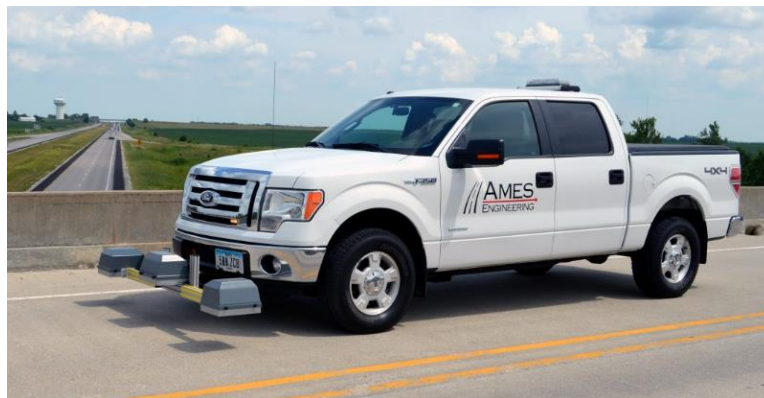
Figure 3. High Speed Inertial Road Profiler (11).
