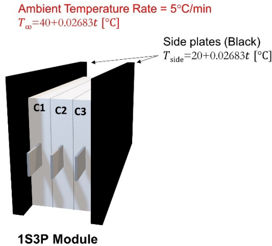
Figure 30. Schematic of a 1S3P module used for thermal ramp experiments and simulations
