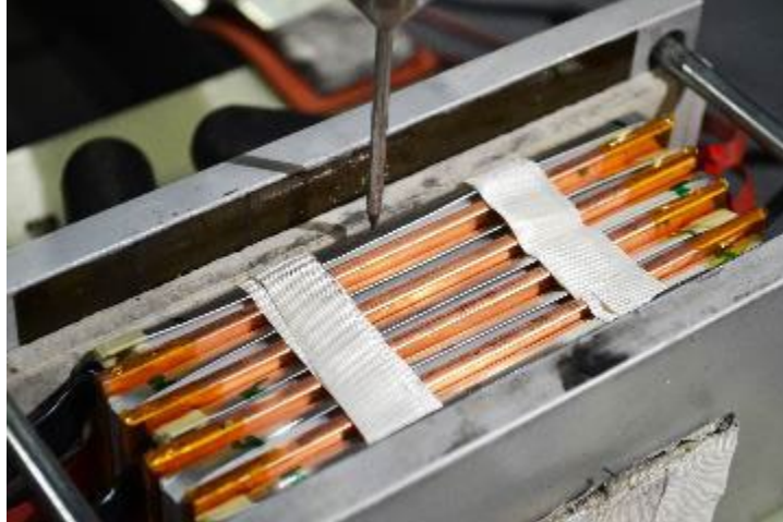
5-cell pack with aluminum or copper spacers between cells
