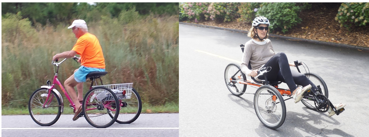
Figure 37. Standard Adult Trike with Basket (left); Recumbent Trike with Two Front Wheels (right)
