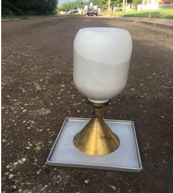
Figure 79. Sand cone compaction test on base layer in the field
