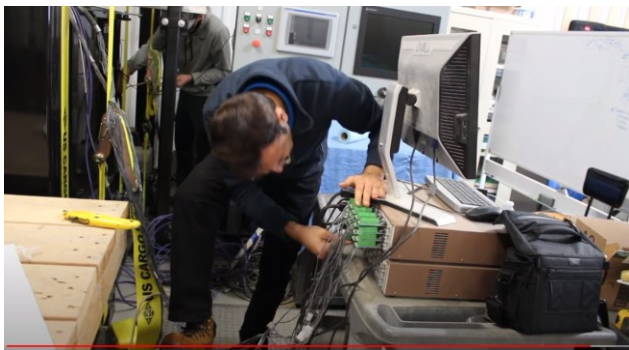
Figure 17. Surface layer preparation steps: a) place a plastic cover layer on top of the aggregate, b) adjust the loading plate on the center of the aggregate layer, c) place the steel layer on top of the plastic cover layer, d) adjust the sensors, and e) set up the strain gauge data acquisition system
