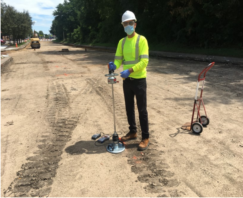
Figure 76. LFWD test on top of the subgrade layer in the field
