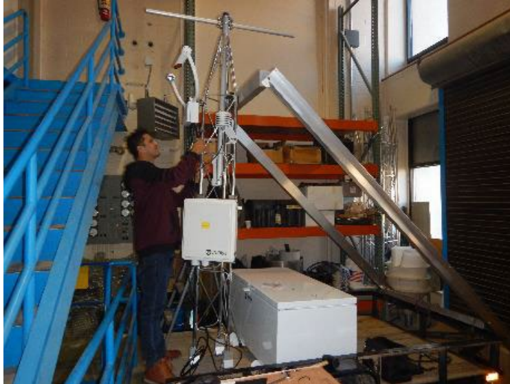
Figure 9: Assembled high-frequency wind monitoring system in the UW Water Resources Lab
