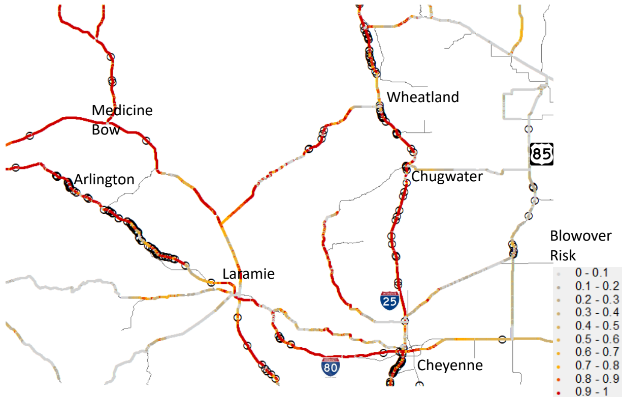
Figure 51: Estimated blow over risk at the historical maximum wind on the highway network of southeast Wyoming based on the WRF simulation. Black circles denote historical blow over crash sites.
