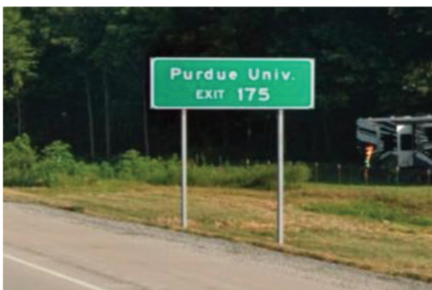
Figure 5.3 The close proximity of the Exit 175 sign to Exit 172 can confuse drivers about which exit they are taking (Google, 2019c).
