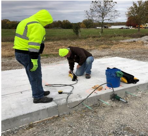
Figure 5 - Physical tests technicians operate the 12-ton hole-ram (left). The tie-bars are threaded so the ram can be fastened to the rebar. The ram is ready for testing (right).
