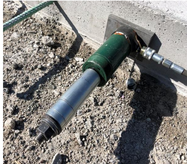
Figure 5 - Physical tests technicians operate the 12-ton hole-ram (left). The tie-bars are threaded so the ram can be fastened to the rebar. The ram is ready for testing (right).
