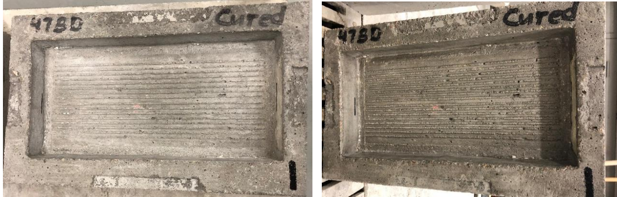
Figure 8 - B1 before testing (left) and after 85 F-T cycles showed no scaling.
