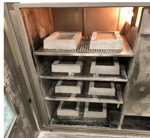
Figure 3 - The ponding blocks were subjected to F-T testing in the environmental chamber.
