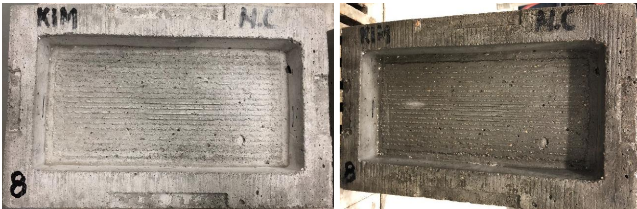
Figure 19- B8 before testing (left) and after testing showed light sign of scaling after 85 F-T cycles.
