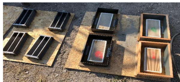
Figure 2 - Forms for T380 Mini-prisms (left) and forms for ponding blocks ready for casting.
