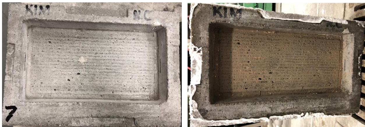
Figure 16 - B7 before testing (left) and after testing showed severed signs of scaling after 85 F-T cycles.
