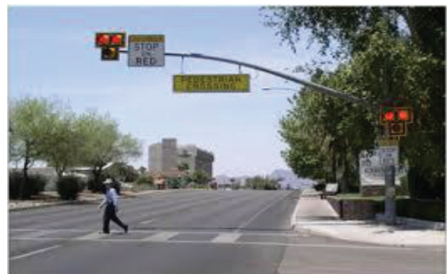
Figure 8.10 Pedestrian hybrid beacon (Source: Michigan Complete Streets Coalition, 2013).
