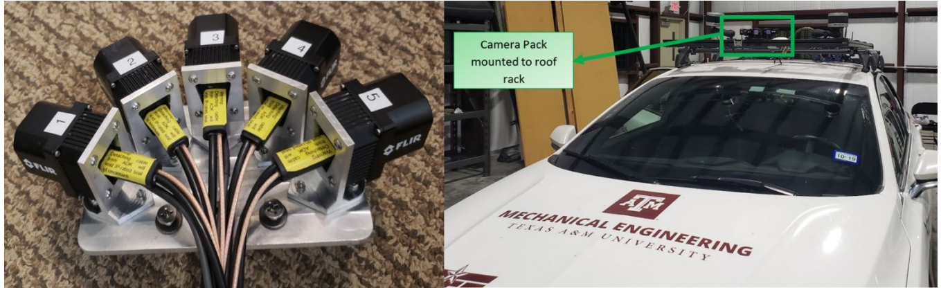
Figure 4: Machined product and mounting location.
