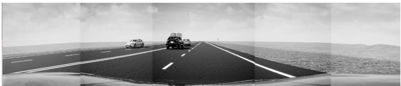
Figure 9: A screenshot showing stitched video, as seen through simulated cameras, from the ego vehicle.
